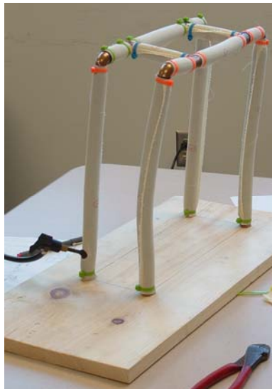
Figure 8: Air Beam Structural Model
