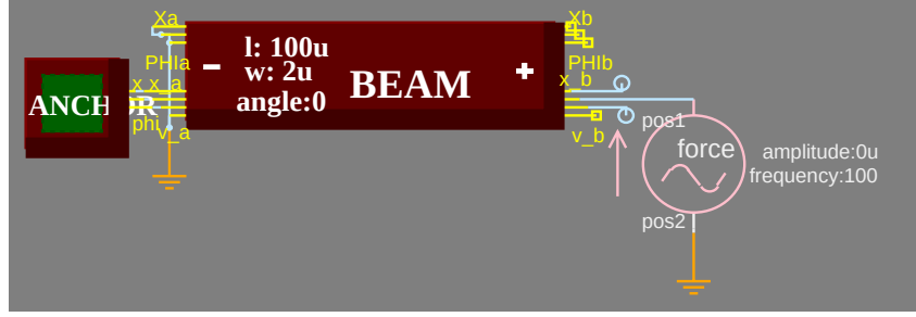
Figure 18. Schematic representation of 100μm long by 2μm wide cantilever beam with AC force source actuating it in the y-direction.
