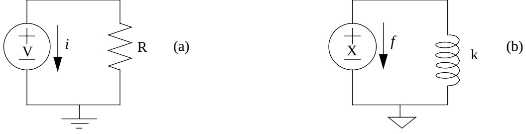
Figure 4. (a) Voltage source connected to a resistor, R . V defines the voltage across the source, while the extra through variable, i , defines the current through the source such that the voltage is maintained. (b) Position source connected to a spring, k . X defines the position across the source, while the extra through variable, f , defines the force through the source such that the position is maintained.
