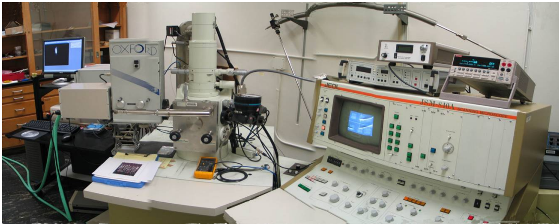
Figure 6. JEOL 840A with Cathodoluminescence and Optical Microscope
