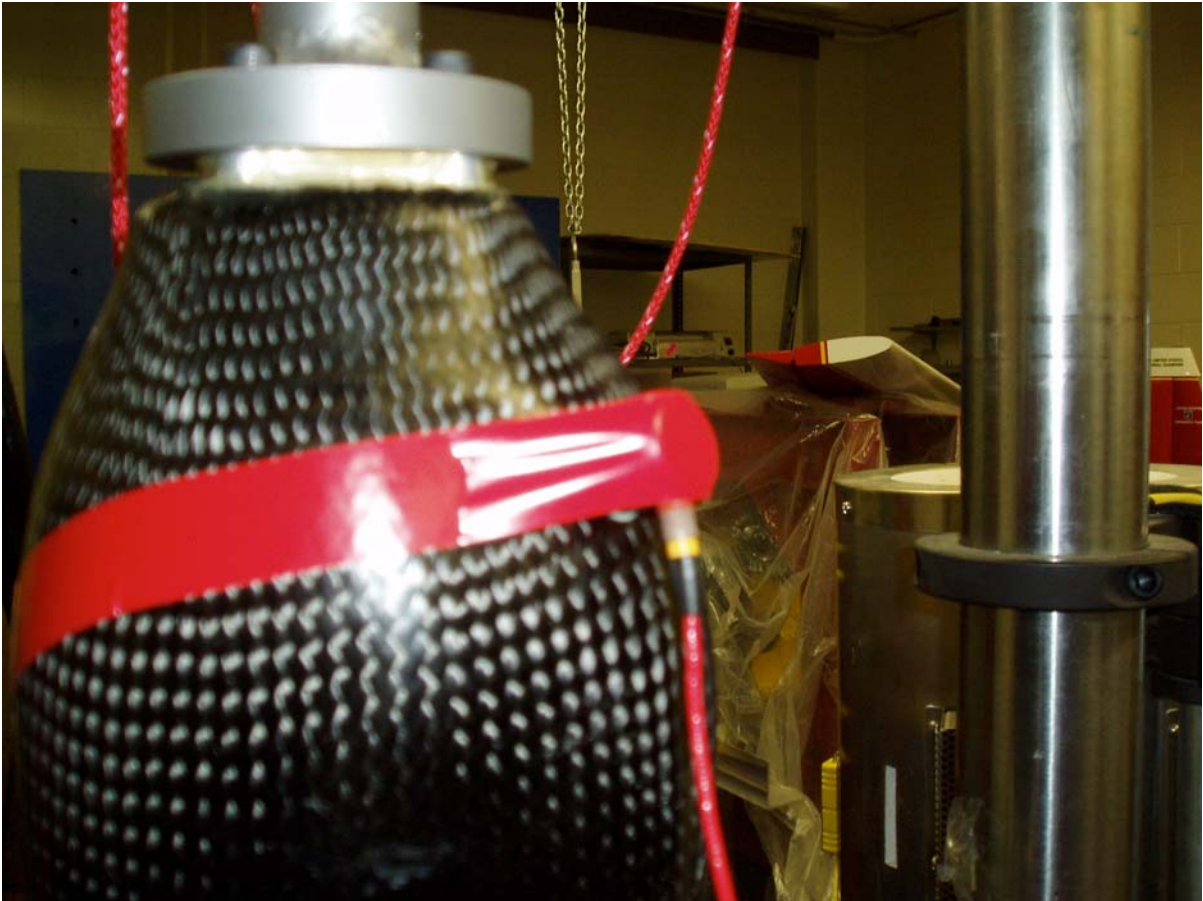
Figure 4. Acoustic emission sensor placement.
