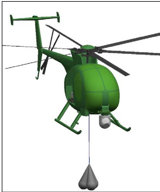
Figure 4. ULB with external hook sling load (From: Cerchie et al., 2008)
