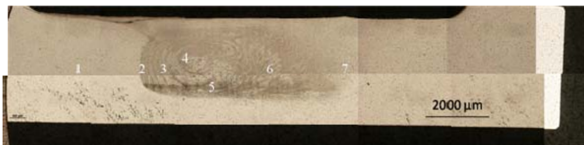
Figure 11. Low magnification montage of as-processed AA5083 showing a stir zone created by FSP at tool rotation speed of 800 rpm and traverse rate of 76.2 \text{ mm min}^{-1} . The stir zone is identified by the grain refinement and flow pattern. The numbers show the sites of optical micrographs.
