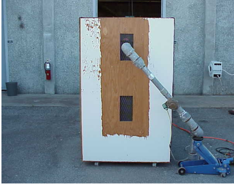
Figure 27. Panel Covering Inlet of Transonic Compressor Rig with Upper Section Steam Injection Pipe Location
