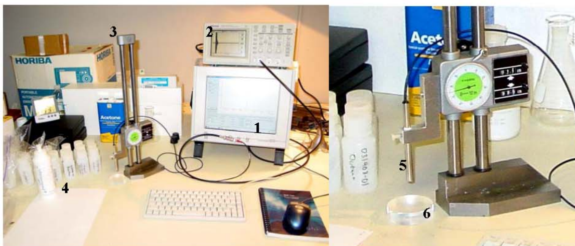
Figure 26: Setup for Gel Sound Speed Measurements (1) DP 2000 Ultrasonic Doppler Velocimeter / Pulse Generator, (2) Tektronics TDS-210 Digital Oscilloscope, (3) Dial Caliper, (4) Gel Samples, (5) Ultrasonic Probe, and (6) Plexiglass Disk
