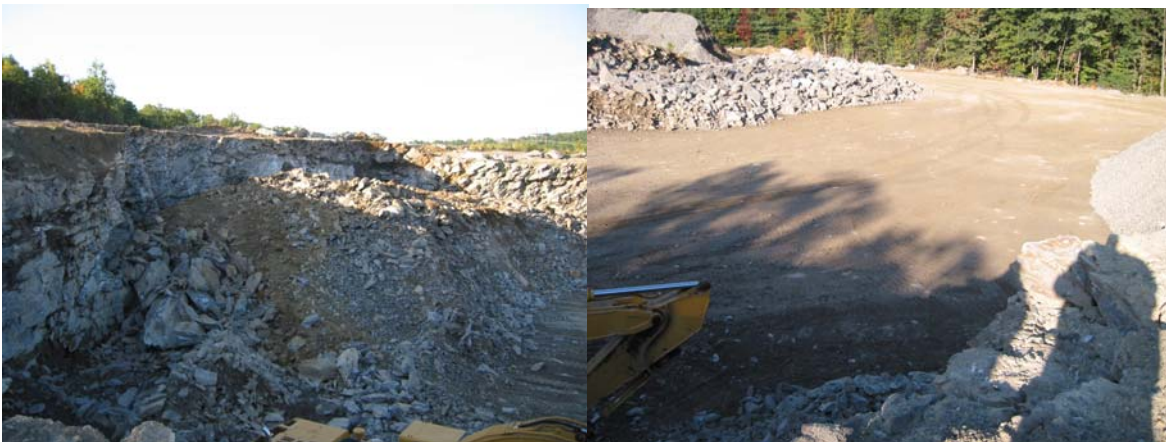
Figure 17. a) Fractured rock from a production shot at a quartzite mine in Leominster, Massachusetts. b) Entrance to pit where explosion tests were to be conducted. The rock below the basal level of the pit is undamaged by previous explosions.
