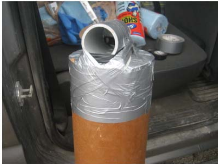
Figure 64. COMP B charge and the tube taped on to hold the detonator.
