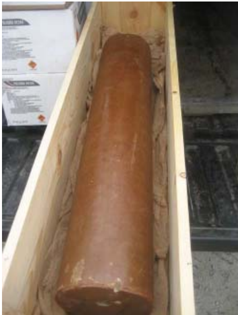
Figure 64. COMP B charge and the tube taped on to hold the detonator.
