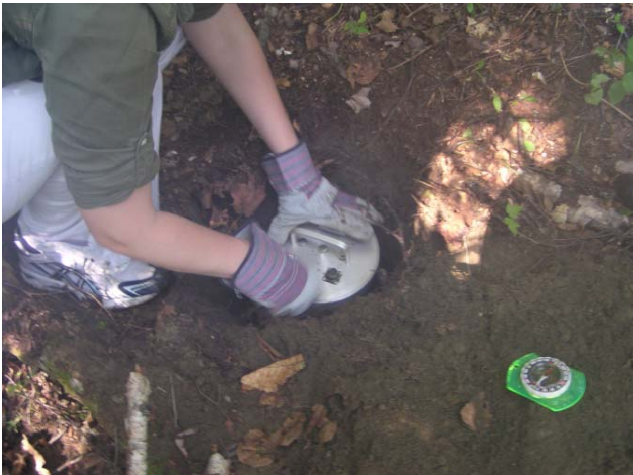
Figure 60. Example of orienting to true north and leveling an L4-3D sensor on the NE line.
