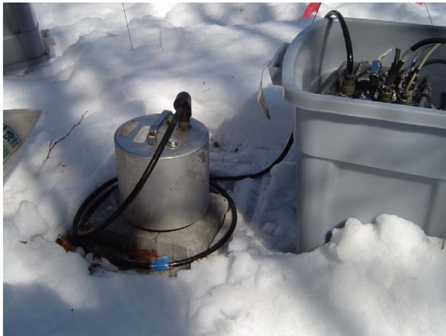
Figure 38. Temporary short-period seismic station FHL consisting of an L4-3D seismometer set up on a stone pad.
