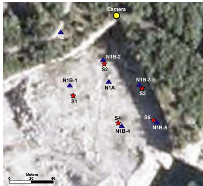
Figure 54. Test site station N1 (blue triangles) and shots (red stars). N1 consisted of two Endeveco accelerometers. N1A remained stationary for all 5 shots, while N1B moved to be less than 5 m from each shot. Station N2 and the camera are also shown on a hill overlooking the test site. (Google Earth Background)
