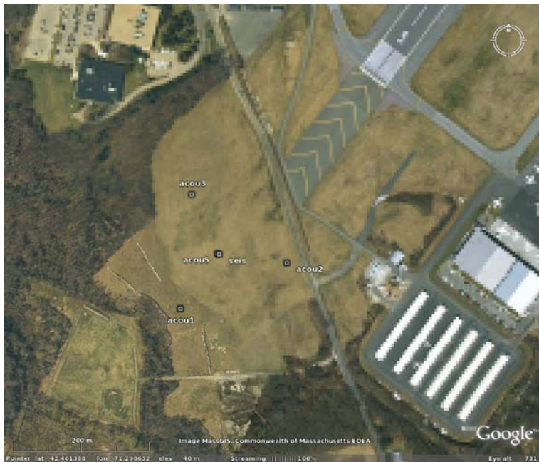
Figure 28. Google Earth image showing the locations of the seismo-acoustic array in relation to Runway 5 at Hanscom Field. The seismic instrument is co-located with the central acoustic element acou5.
