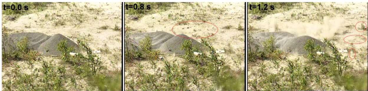
Figure 71. Digitized still images of the Shot 1 detonation. Note the two fractures developing after 0.8 s and the further fractures after 1.2 s in the red ellipses.
