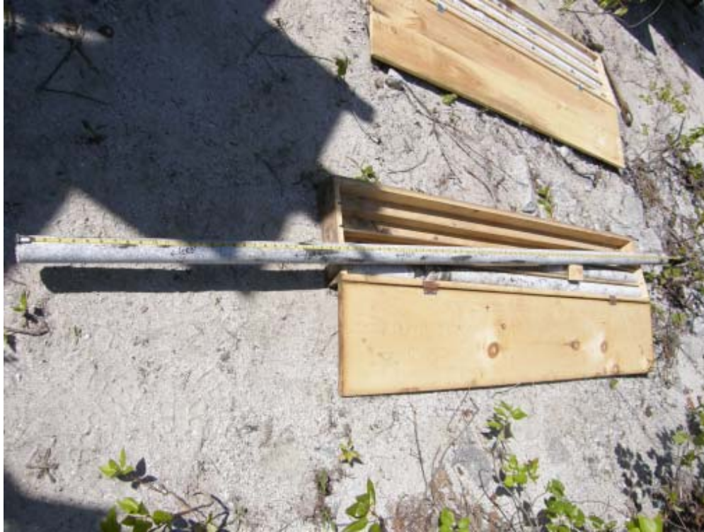
Figure 95. Example of unfractured core taken from the test site.
