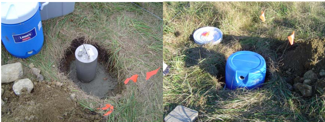
Figure 30. Placement of seismometer on concrete surface before being enclosed by the insulating cooler.
