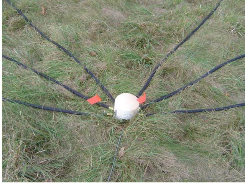
Figure 29. A Chaparral acoustic sensor with attached soaker hoses for wind noise reduction.
