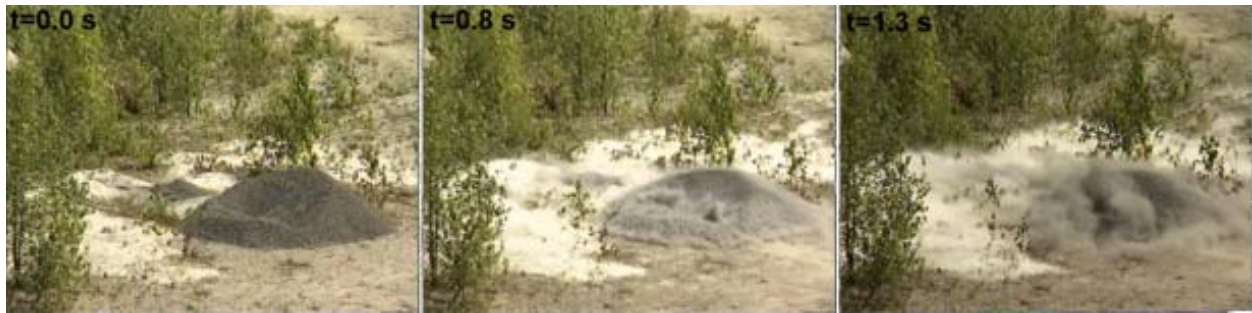
Figure 75. Digitized still images of the Shot 4 denotation. This shot produced significantly more dust than Shots 1-3. There may be small amounts of gas release in the gravel pile after 0.8 s, but there were no large fractures observable on the video like for Shots 1 and 2.
