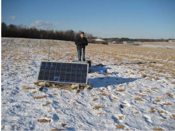
Figure 31. Solar panel that powers the HANS seismo-acoustic array at Hanscom Air Force base.
