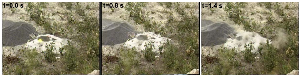
Figure 73. Digitized still images of the Shot 2 detonation. Three fractures develop in the white granite floor at 0.8 s and a larger opening releases a plume of gases to the right of the floor at 1.4 s.
