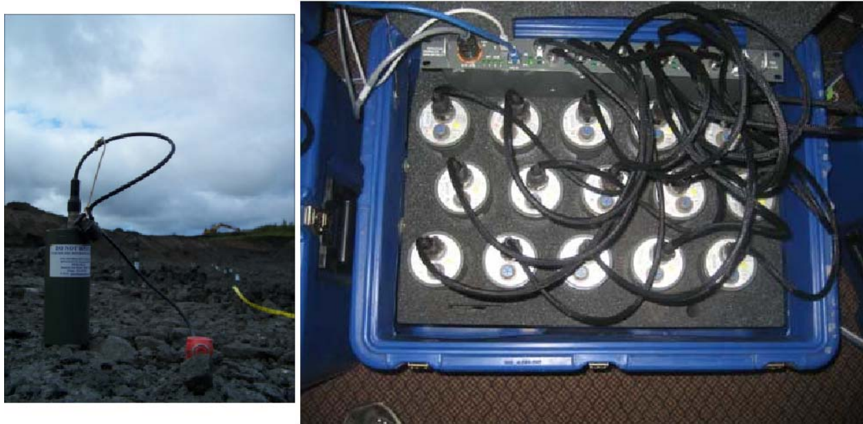
Figure 61. (Left) RT-125 “Texan” seismic recorder and attached 4.5 Hz vertical spike geophone (orange). For the experiment, the recorder was placed in a plastic bag, laid on its side in a trench, and everything was buried. (Right) Texans in their carrying crates being programmed prior to deployment.
