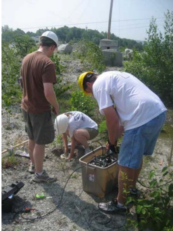
Figure 56. Example of near-source instrument installation. Katherine Murphy levels and orients a TerraTek accelerometer to true north while Sam Huffstetler installs the Reftek 72A-08 digitizer and battery.
