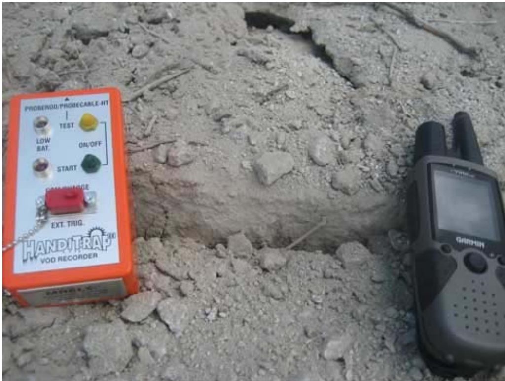
Figure 72. Largest crack generated by Shot 1.
