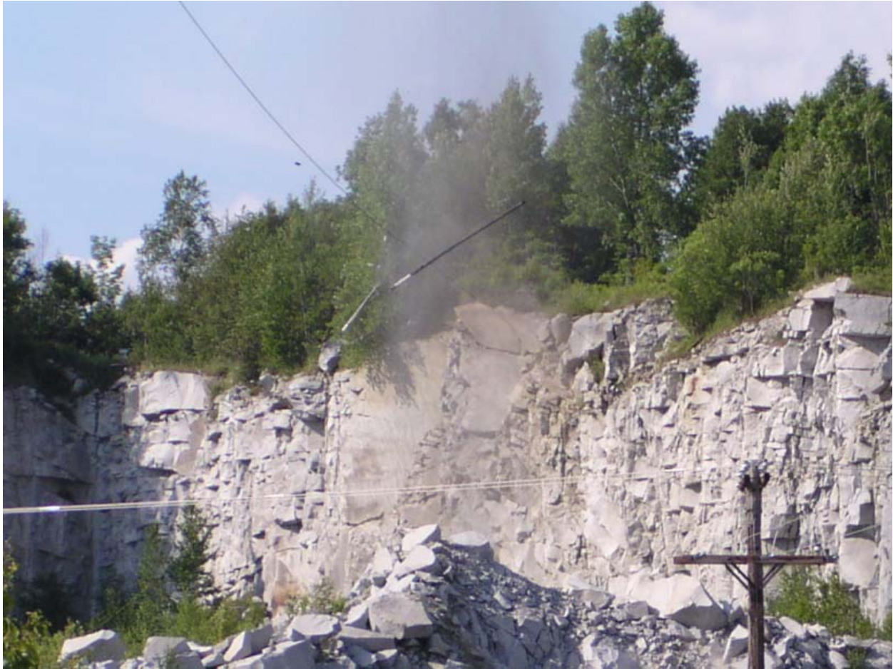
Figure 78. PVC pipe breaking on guy line during free fall after being ejected from a nearby borehole during Shot 5.
