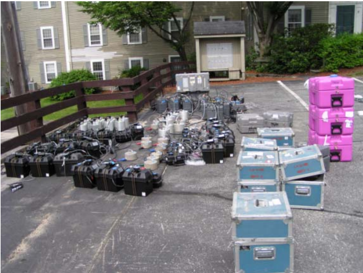
Figure 101. Huddle test in the Weston Geophysical parking lot prior to the experiment.
