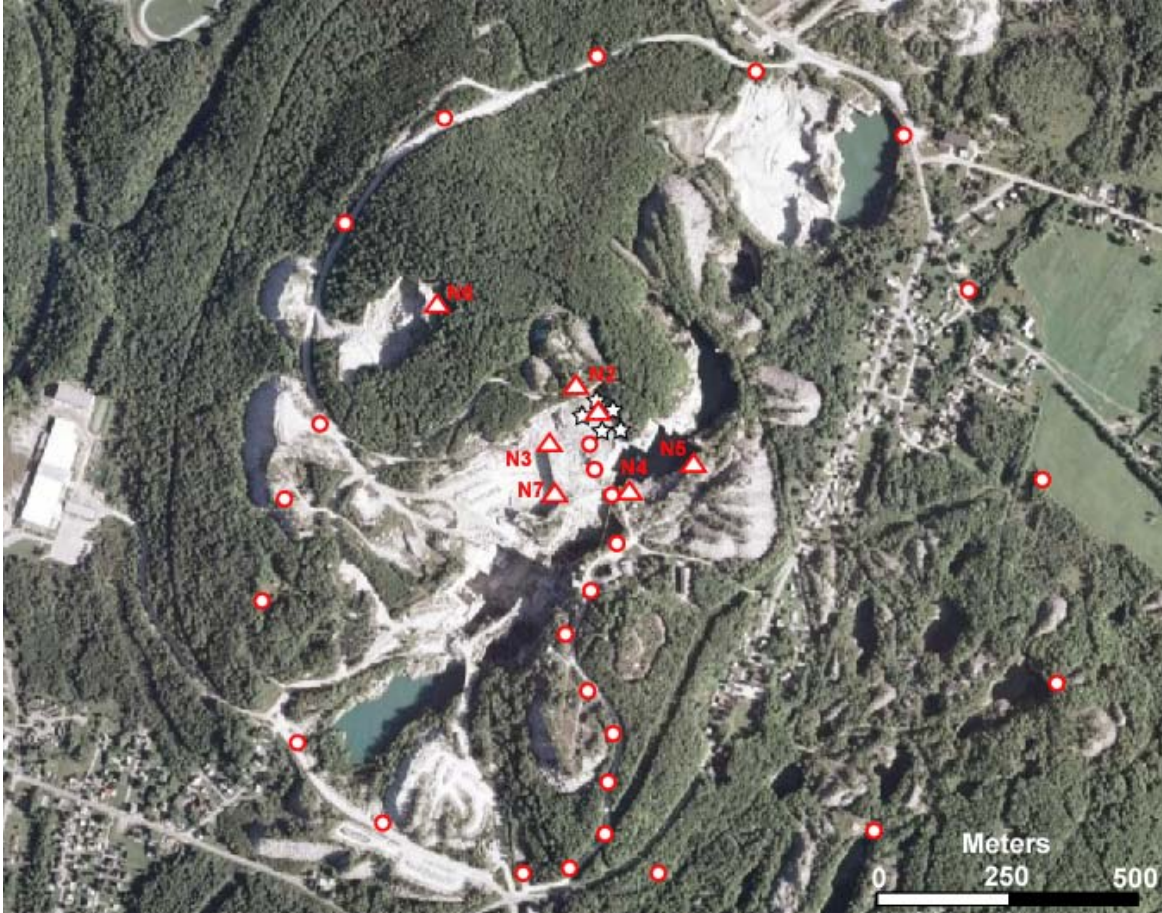
Figure 55. Near-source stations N1-N7 (white triangle with red outline) and Texans ‡ NT01-NT27 (white dot with red outline). N1 consisted of two sensors, one of which moved for each shot (Figure 54). The shots (white stars with black outline) can be seen in the middle of the image. (Google Earth Background)
