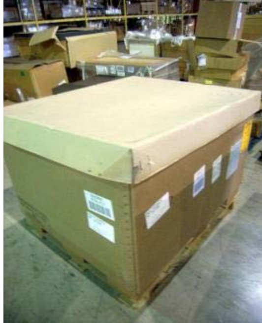
Figure 2. A triwall (depicted above) allows helicopters to move medium size cargo without eliminating passenger seating.
