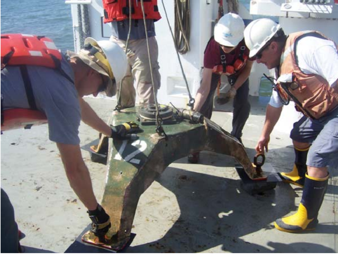
Figure 4. Recovery of a pressure sensor (PA) tripod during the final recovery cruise of MUDEX. The pressure sensor is fitted to a fiberglass tripod equipped with lead feet to ensure stability on the ocean floor. The small cylinder to the right of the pressure sensor is an acoustic pinger that helps locate the instrument.
