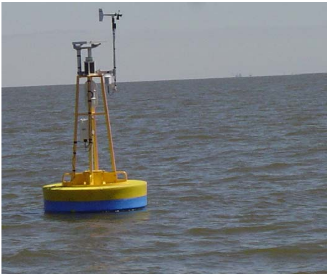
Figure 10. Meteorological buoy deployed by WHOI during MUDEX. The anemometer is 3m above sea level and is the tallest sensor attached to the buoy. (From Dr. Janet Fredericks at WHOI)
