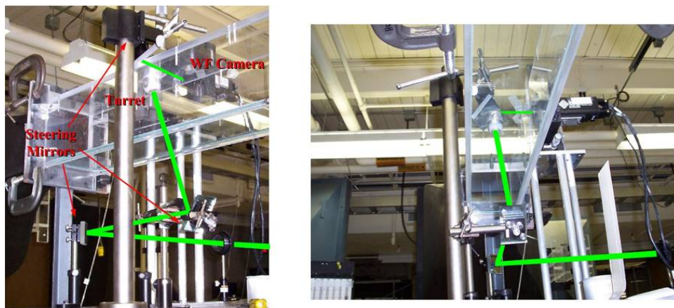
Figure 21: Optical set-up to measure 2-D wavefronts.
