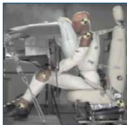
The AmSafe Aviation Airbag's four-point configuration used for GA aircraft.
