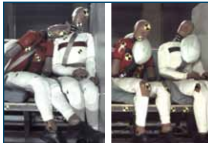
A tubular three-point restraint compared with a standard three-point restraint in a lateral impact.
