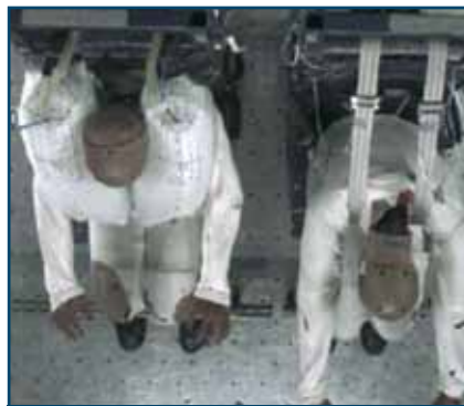
The tubular AmSafe Aviation Airbag four-point restraint compared to a standard four-point restraint.
