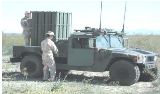
Figure 6. NLOS-LS Box Containing 16 Slots
