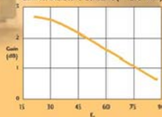
Gain vs. groundplane size (25 mm patch)
