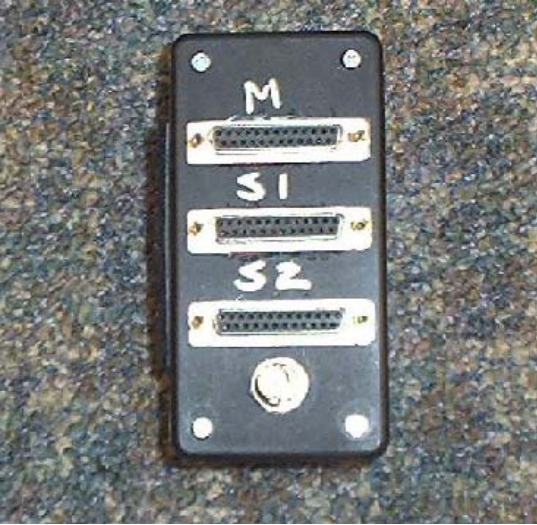
Fig. 2: A fabricated box that handles genlocking and data locking through parallel port connections.
