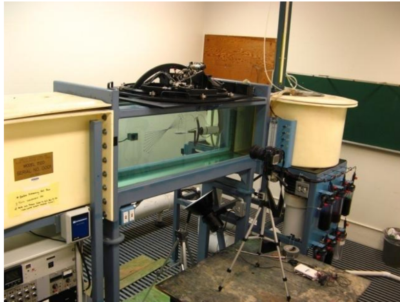
Figure 6. NPS 15" x 20" Flow visualization water tunnel
