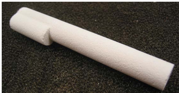
Figure 2: The Gen3.1 iteration of the porous separator is shown which was fabricated in house to a porosity of great then 60%
