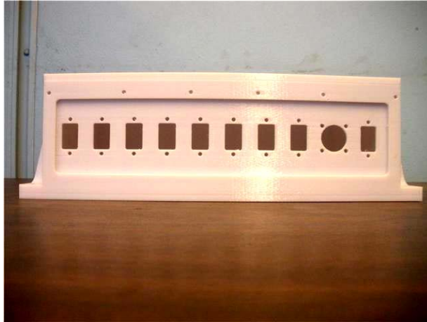
Figure 15. 3D Model Final Prototype Front Face Plate Connector Cutouts
