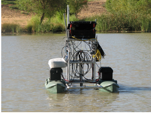
Figure 10: The aquatic Networked Infomechanical System (NIMS-AQ) [16] for environmental monitoring.
