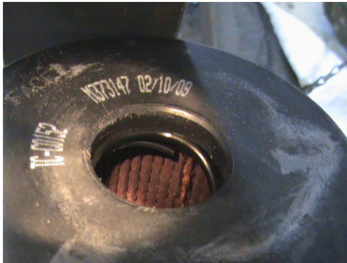
Figure 6. Torn o-ring in PecoFacet end cap
