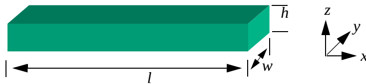
Figure 2-2: A cantilever beam.
