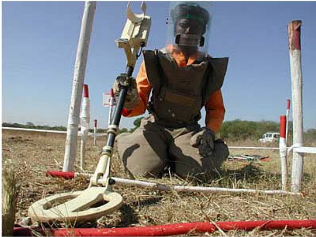
Figure 1. EMI detector for humanitarian demining use.
