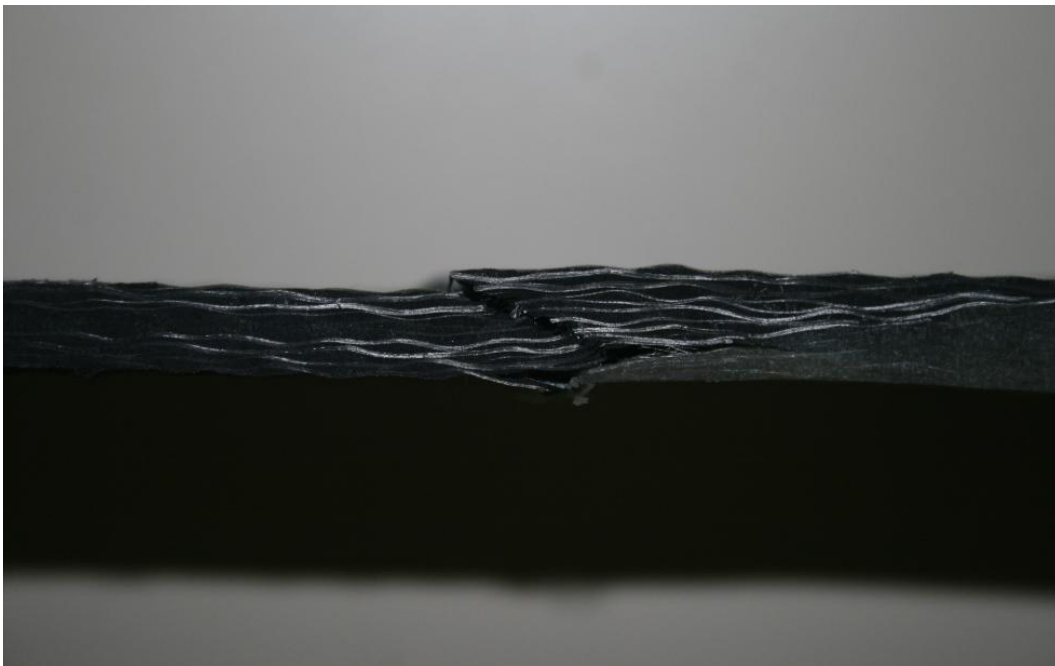
Figure 9. Compressive Tests–Carbon Side Failure
