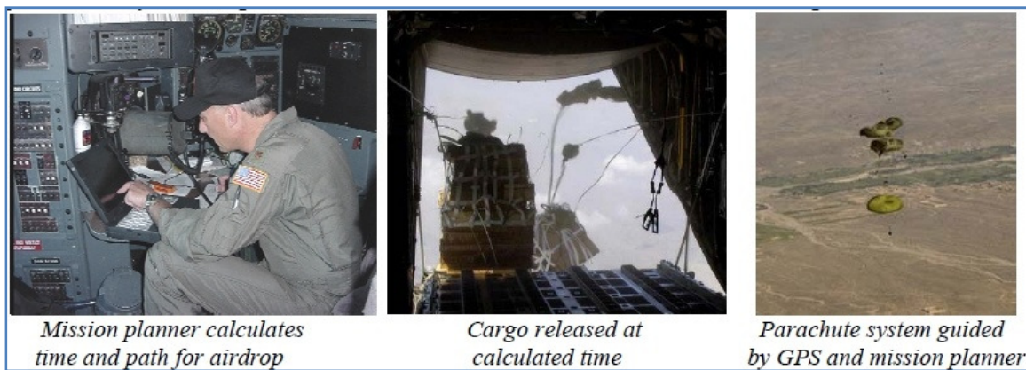
Figure 7 - JPADS enables standoff precision airdrop using guided parachutes[26]
