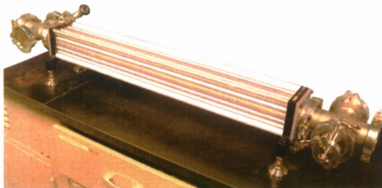
Figure 2. Second vacuum cavity. The length is 750 mm. The Swagelok port and top windows have been replaced by vacuum tees at both ends of the aluminum profile.
