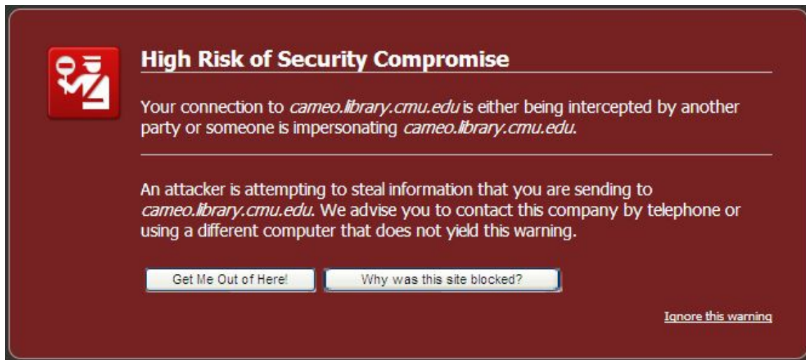
Figure 8.8: This newly designed SSL warning clearly states the threat it is guarding against, the consequences of ignoring it, and how to mitigate the risks.
