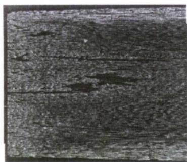
Dark-field image of oxidation
