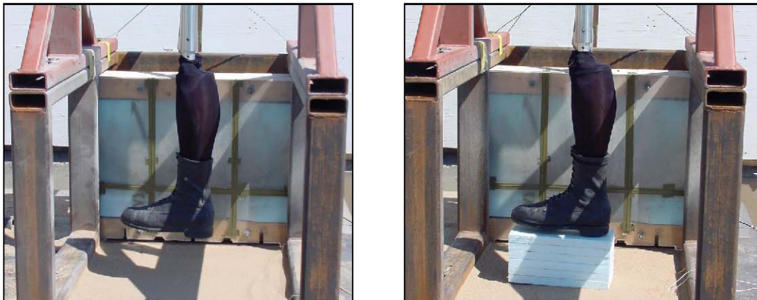
Figure 1. Setup to study the effect of standoff on the level of injury; (left) with an air gap and (right) with Styrofoam® inserted.
