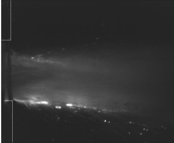
Figure 8: Leaning sprays are not attached to the injector wall at the exit of the injector (shown by lines).
