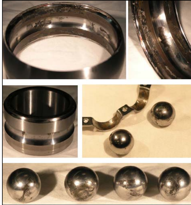
Figure 12. Photographs of corrosion damage to bearing 019-ARL-RS after post-test disassembly.
