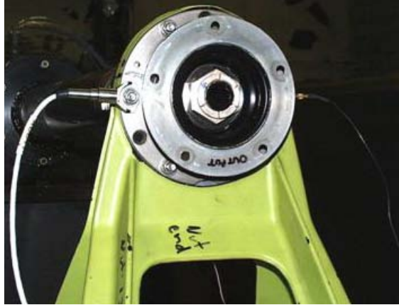
Figure 3. Orientations of two accelerometers attached to the hanger assembly
