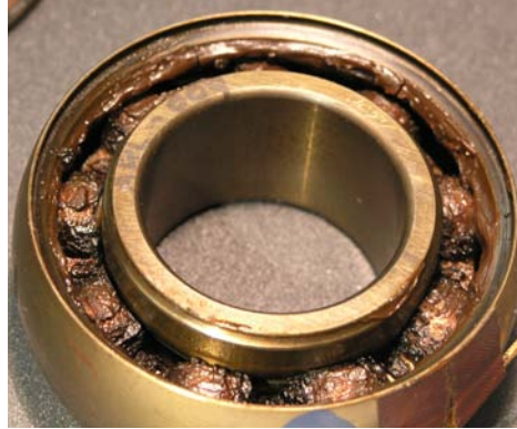
Figure 17. Grease appearance after 1600 hr of elevated temperature (accelerated life) operation.
