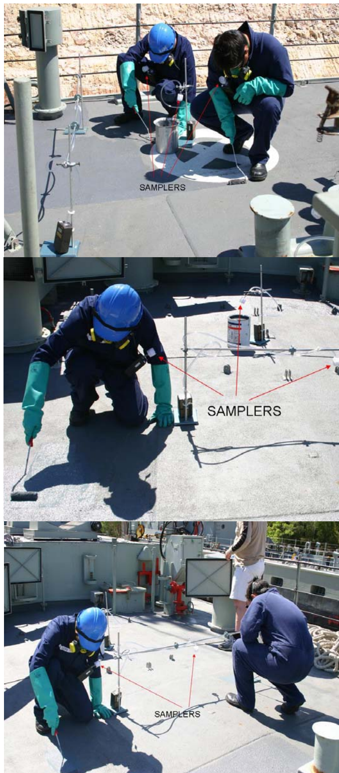
Figure 4: Painting trial, HMAS CESSNOCK, Darwin, showing locations of air sampling of personnel and down wind
