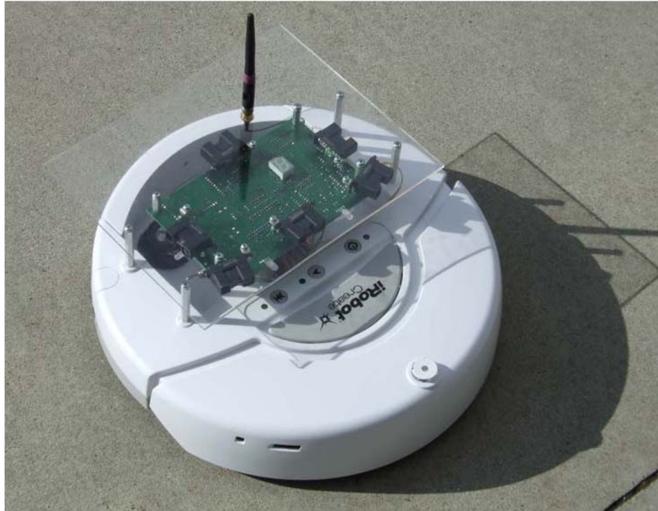
Figure 1.2: Autonomy Lab Chatterbox robot pre-production prototype.
