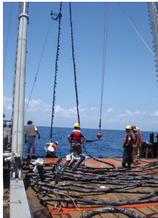
Figure 44 HGMS Array Cable “Bite” Deployed by the A-Frame. Array Flaked on Deck
