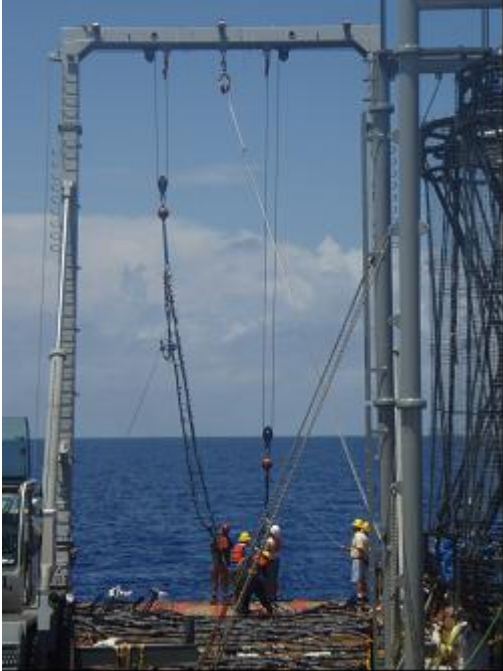
Figure 38 HGMS 45-ft Tall A-Frame
