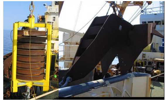
Figure 5 Bruce and Clump Main Mooring Anchors
