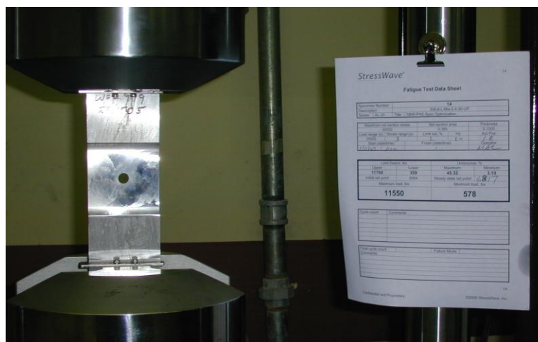
Figure 36. Typical Constant Amplitude Test Setup
