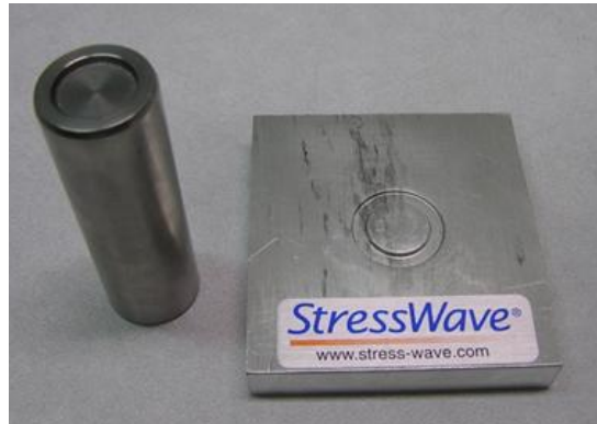
Figure 3. StressWave Indenter and Corresponding Dimple (for a 1 inch CW hole)
