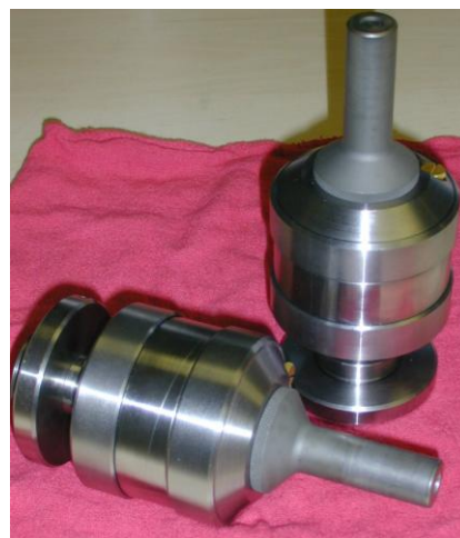
Figure 46. Proof of Concept Hydraulic Pressure Foot End Effector
