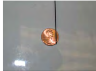
Figure 1.0. First generation needle compatible fiber probe (next to penny to demonstrate size). Imaging resolution using the system has been experimentally demonstrated to be < 10 \mu\text{m} .
