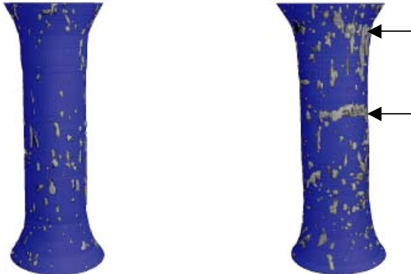
Fig. 15. Three-dimensional micro-CT reconstructions of the entire gauge section (2.5 mm diameter) in a (left) unloaded control specimen and (right) specimen loaded in cyclic uniaxial tension. Arrows highlight regions of BaSO 4 staining characteristic of fatigue damage and/or propagating microcracks.
