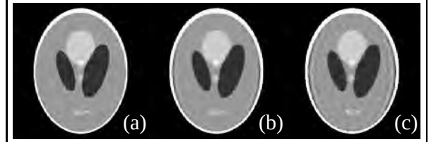
Figure 4: The true image (a) and images reconstructed by use of (b) proposed TV algorithm and (c) original TV algorithm after 200 iterations. Notice that these two images represents the intermediate images after certain iterations. The display gray scale is [0.9, 1.1] .
