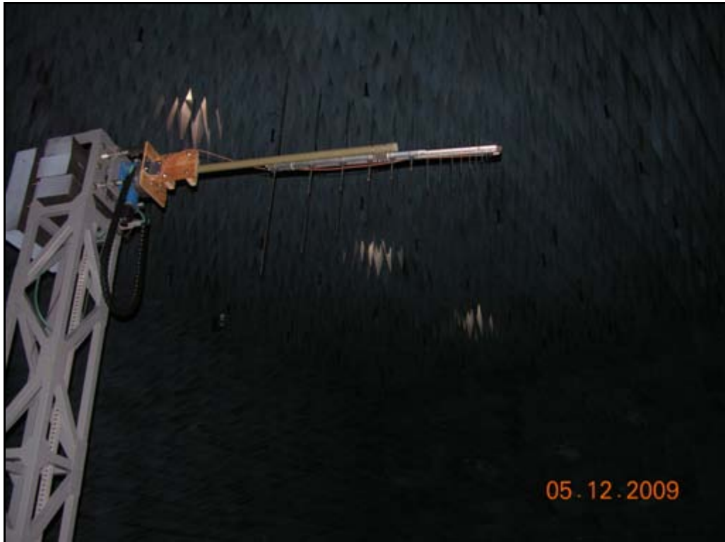
Figure 2. Log periodic antenna mounted with a tubular fiberglass pole.
