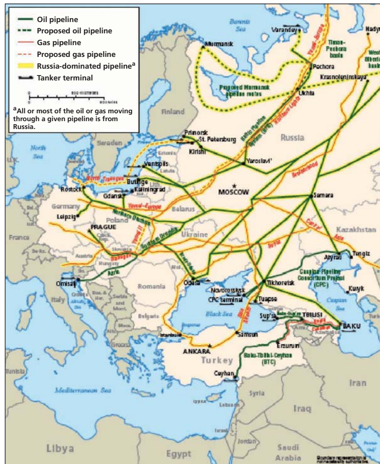
Figure 3.1 Russian Oil and Gas Pipelines to Europe
