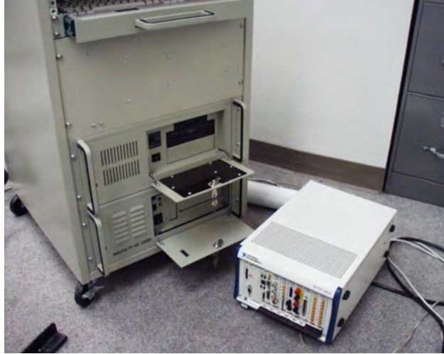
Figure 1: Comparison of older, in-house data acquisition system (left) with commercial solution (right)
