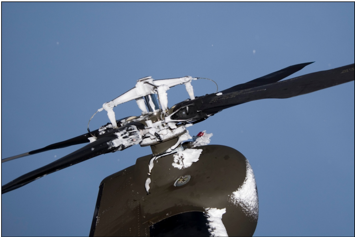
Figure XX. Ice Accretion on Tail Rotor Hub
