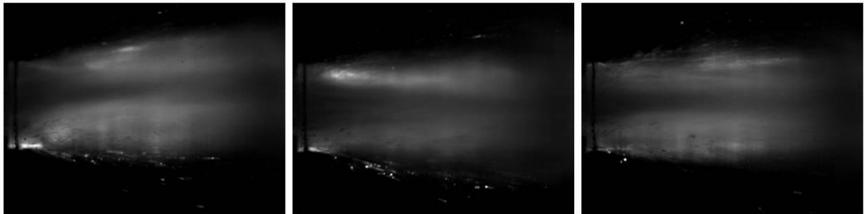
Figure 4: Three frames of video (~1.33 ms apart) show the typical path of an oscillating spray.
