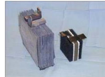
Conventional lead-acid vs. advanced lead-acid
