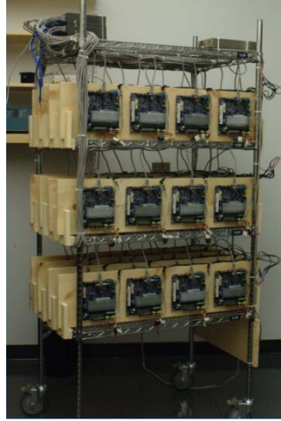
Figure 9: Photo of Wireless Ad-hoc Network Consists of 32 Computation Nodes, Each Running DWARF
