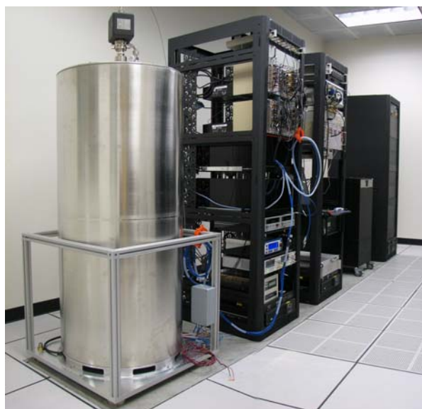
Figure 4. Initial install of Rb fountain with hydrogen maser.
