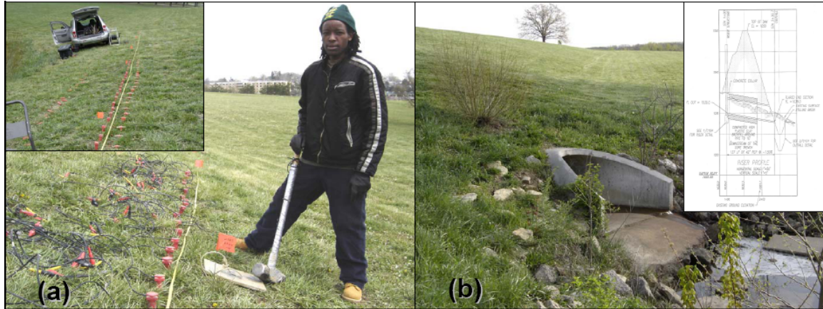
Figure 1: (a) 4.5 Hz geophone array over spillway tunnel at a Ber Juan Park, Rolla, MO.: Graduate student Wamweya uses a sledge hammer source to generate surface wave energy. (b) Design blueprints and on-site measurements of the Ber Juan spillway pipe are compared to the geophysical interpretations to assess the reliability of automated interpretation methods.
