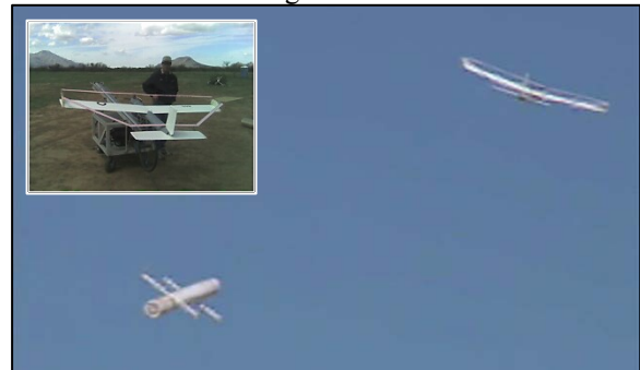
Figure 7. Configuration One - Airborne gradiometer with the Silver Fox mounted transmitter and a towed, air core gradiometer. Insert shows transmitter.
