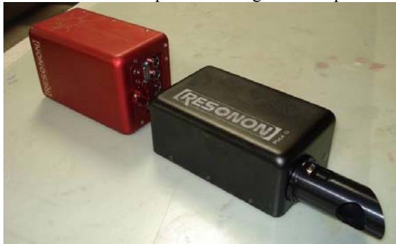
Figure 6. Hyperspectral imager produced by Resonon for the Silver Fox UAV..
