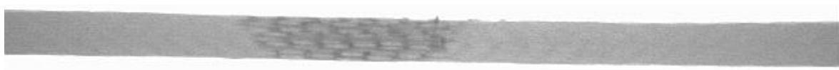
Figure 10. Side view of sample with alloying from real time X-ray (Creep test at 110.5 MPa and 1204°C for 1269 hours)
