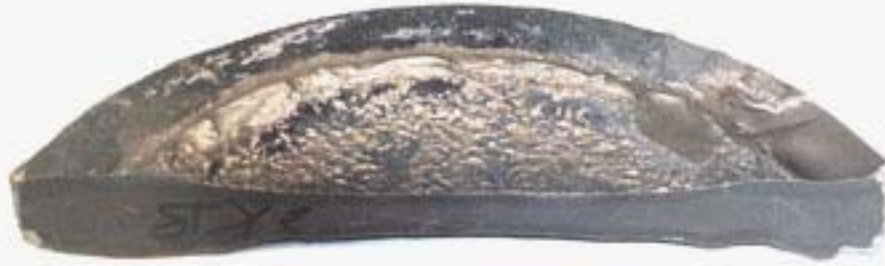
Figure 2: An 03K pancake segment showing the dog-bone shape cross-section
